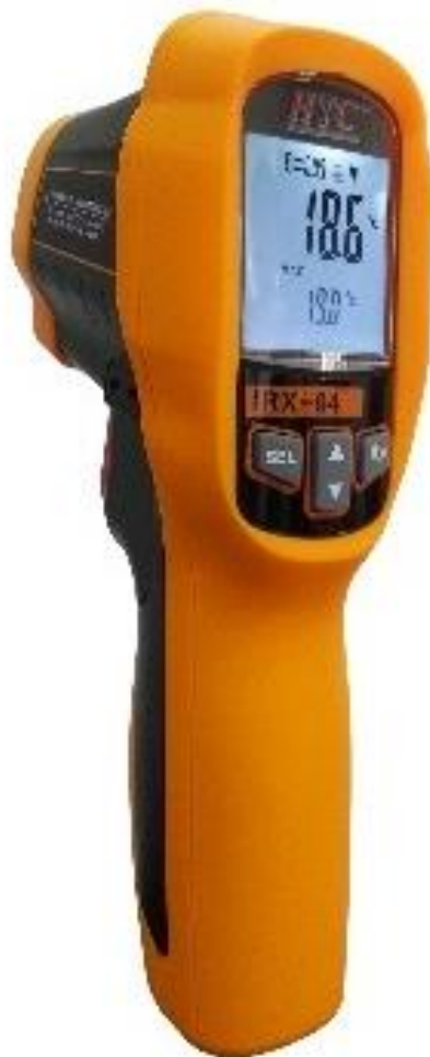
Picture 5 HTC IRX 64 Infrared thermometer
