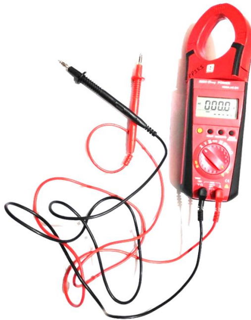
Picture 3 RISH POWER CLAMP 1000 A/400 A AC-DC
